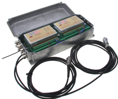
2 of PCH 1073 in IP67 casing
